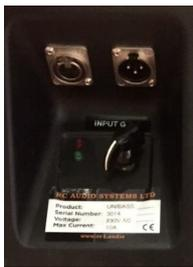
Audio input is via a balanced XLR connector, and this is directly linked to an XLR output connector so that the input signal can be linked to other units.
