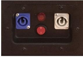
Power in is via a 20amp "Powercon" inlet connector.
