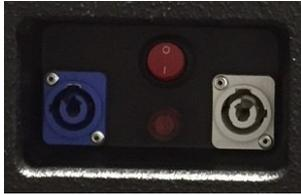
Power in is via a 20amp "Powercon" inlet connector.
