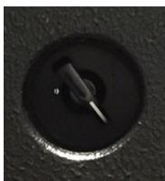
There is a separate recessed adjustment for the Leveliza threshold.
