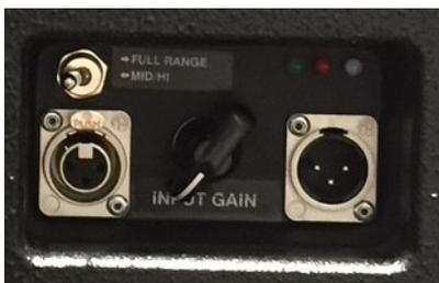
Audio input is via a balanced XLR connector, and this is directly linked to an XLR output connector so that the input signal can be linked to other units.
