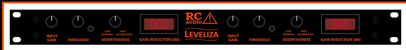
The LEVELIZA is a totally new type of product. It uses a new type of circuit to specifically identify the audibly loudest significant components in a music signal, and then it analyses them over a period of time in order to identify the average perceived loudness of the music. When this average perceived loudness exceeds the set threshold it very slowly and subtly adjusts the system gain so as to try to maintain the average perceived loudness around the threshold.
